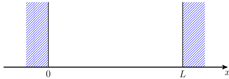
Figure 1: Geometry for the one dimensional Casimir calculation: two perfectly conducting plates separated by a distance L .
